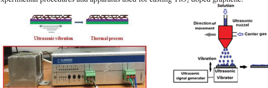
Schematic 1 -Ultrasonic vibration assisted spray coating, ultrasonic vibration equipment, thin film formation mechanism
