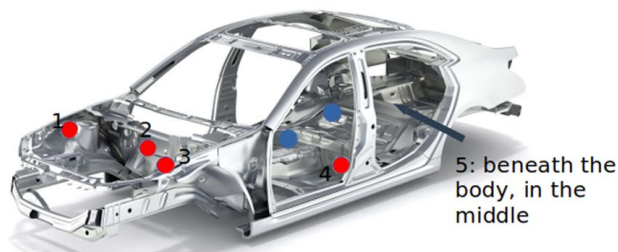
Fig. 2 The locations of vehicle body accelerometers
